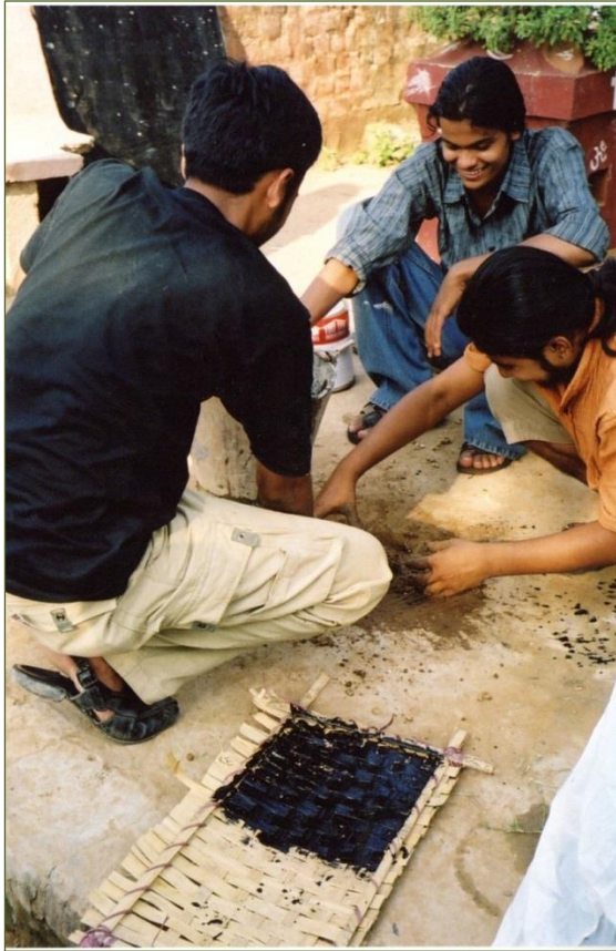
Fig. 9 Manufacturing sandwich panels in a settlement in Ahmedabad, India
