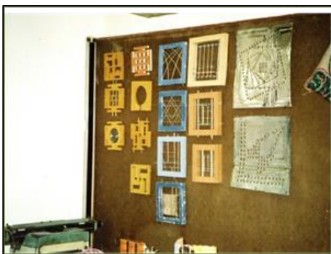
Fig. 7 Translucent panes from various waste products manufactured from municipal solid waste in India
